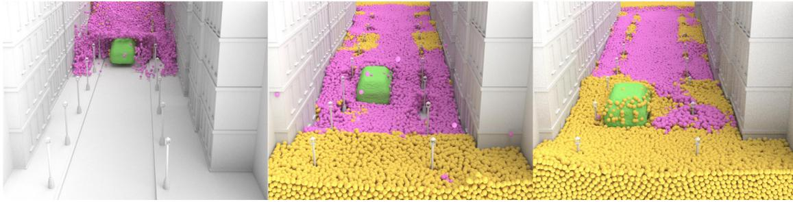
Fig. 10. The result of particle partitioning procedure for rigid body-fluid interaction.
